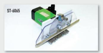
> Cutting machine ST-6065 for the series K-130 (with three-phase motor, two-sided cutting, up to 21 mm / 0.8" material thickness)
